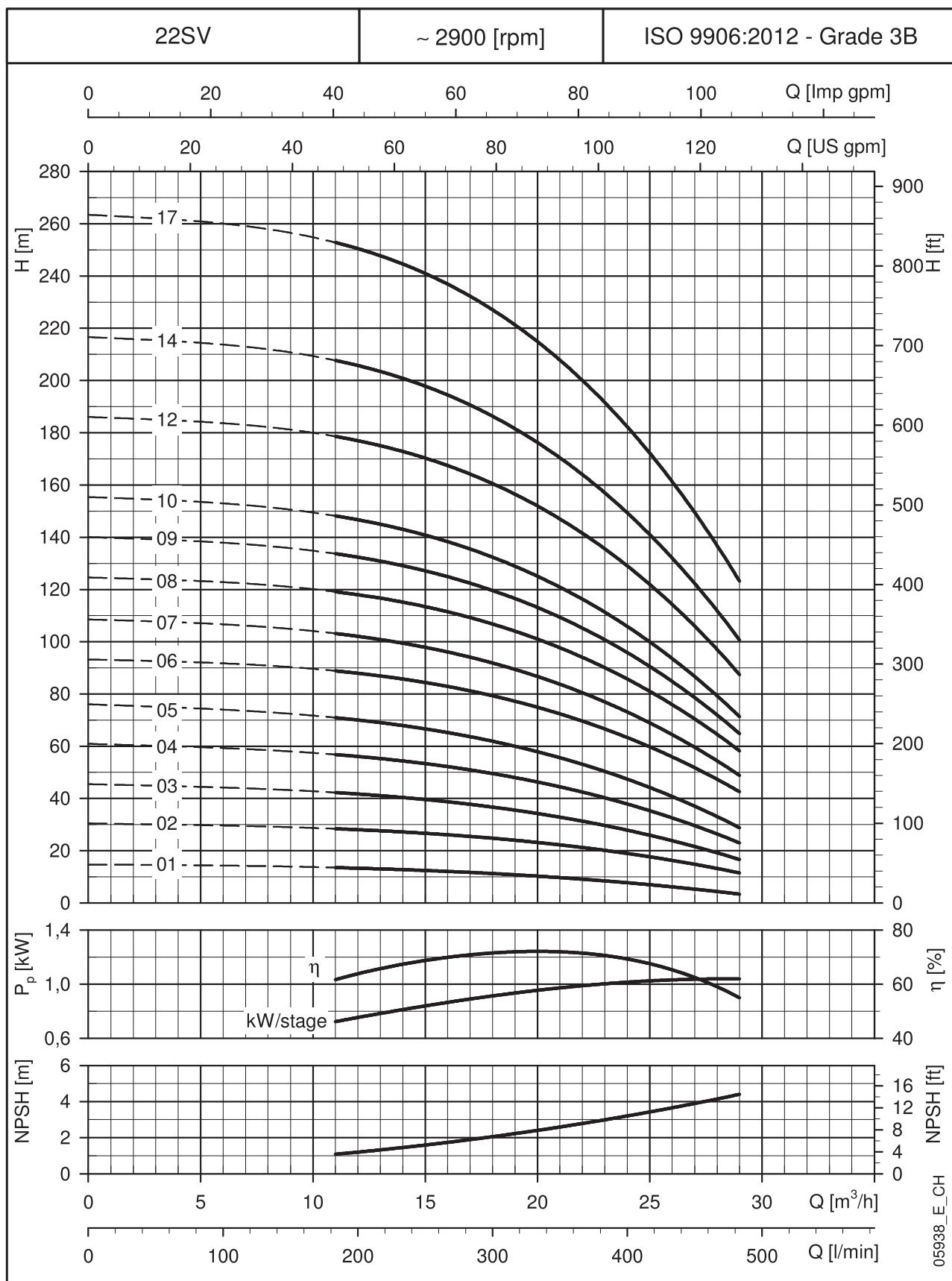
These performances are valid for liquids with density  $\rho = 1.0$  Kg/dm<sup>3</sup> and kinematic viscosity  $\nu = 1$  mm<sup>2</sup>/sec.
